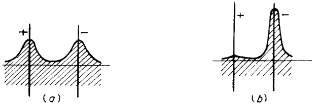
Figure 3. The profile of the dielectric liquid. (a) The first range of voltages; (b) the second range of voltages.
